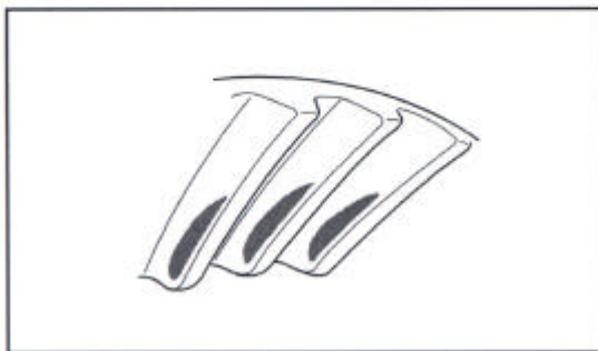
If the pattern is too close to the top land of the gear tooth, remove pinion shims.
