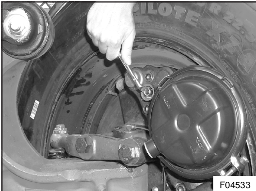
Figure 5: To turn the adjuster stem with a box wrench
