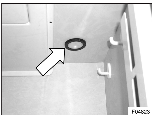
Figure 22: Roof light in lavatory compartment
